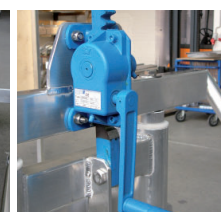
Rack and pinion jack for the height adjustment.
